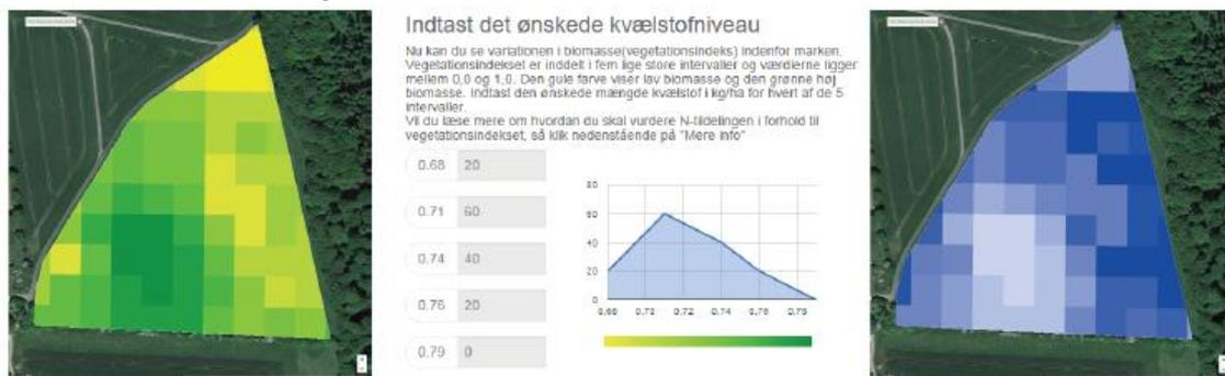
Fig. 1. The green map shows the vegetation index (NDVI) for a field. Yellow = low biomass and green = high biomass. The farmer writes in kg nitrogen per hectare in the 5 levels. The blue map shows then the variable rate application map. Light blue=low amount of nitrogen and dark blue = high amount of nitrogen. The application file can be exported as a shape file. The tractor terminal can read the file and will spread the fertilizer according to the blue map.
